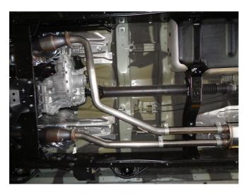
**Step 2.** Begin installation by loosely attaching the Inlet Pipe Assembly to the catalytic converter flange using the OEM hardware. Engage the welded hanger to the rubber insulator.
