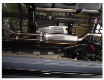
**Step 3.** Loosely attach the Muffler Assembly using the supplied clamps. Engage all welded hangers to the rubber insulators.
