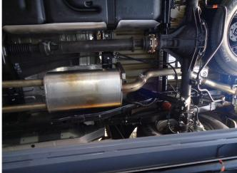
**Step 1.** To remove the OEM exhaust loosen the fasteners at the 2 bolt flange attaching the inlet pipe to the catalytic converter outlet. Working front to rear disengage all welded hangers from the rubber insulators. Also, loosen the clamp after the muffler. Be sure to retain all mounting hardware as it will be needed to install your new MAGNAFLOW system.
