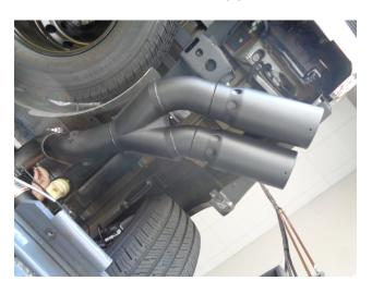
**Step 4.** Install the Tail Pipe Assembly in the same way. Once a final position has been chosen for the new exhaust system, evenly tighten all clamps from front to rear using the torque specifications on page one of the instructions. Inspect all fasteners after 25-50 miles of operation and re-tighten if necessary.
