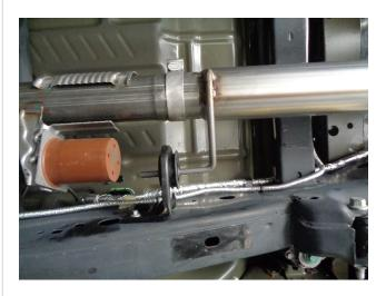
**Step 2.** Install Inlet Pipe Assembly. Loosely fasten it to the DPF outlet using supplied clamp.
