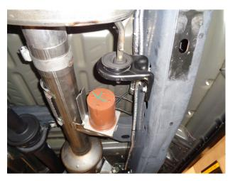
**Step 1.** Working front to rear loosen or remove all OEM band clamps and disengage all welded hangers from the rubber insulators. Be sure to retain all mounting hardware as it will be needed to install your new MAGNAFLOW system. Slide the OEM system off towards the front of the vehicle.
