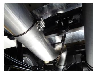
**Step 3.** As you assemble the Extension Pipes loosely locate the Hanger Clamp Assemblies as needed then instal the over axle pipe.
