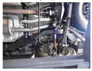
**Step 5.** If you have the MAX version of the Expedition you will need to loosely install the 11.25" Extension Pipe Assembly. Next, loosely attach the Over-Axle Pipe Assembly and the Tail Pipe Assembly using the supplied 3.00" clamps and engage the welded hangers to the OEM rubber insulators. Re-install sway bar.
