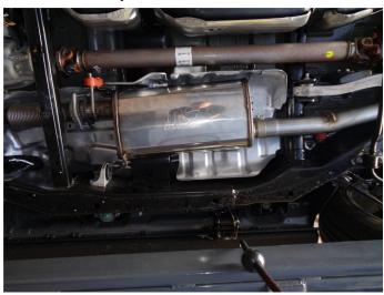
**Step 4.** Begin installing your new MAGNAFLOW system by loosely bolting the Muffler Assembly inlet flange to the flex assembly outlet using the supplied hardware.
