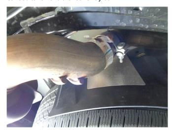
**Step 2.** Next, remove the tail pipe section by loosening the OEM clamp. Disengage the welded hanger from the rubber insulator and remove the tail pipe assembly. Do not discard the or damage the rubber insulators as they will be used to mount the new system.
