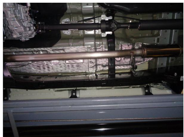
**Step 1.** To remove the OEM exhaust system, you can then disengage the welded hangers from the rubber insulators and remove the tailpipe assembly. Unfasten the clamp attaching the OEM inlet pipe assembly to the catalytic converter. Do not damage or discard the inlet pipe clamp or rubber insulators as they will be re-used to mount the new system. Disengage the inlet pipe assembly hanger and remove the exhaust from the vehicle.
