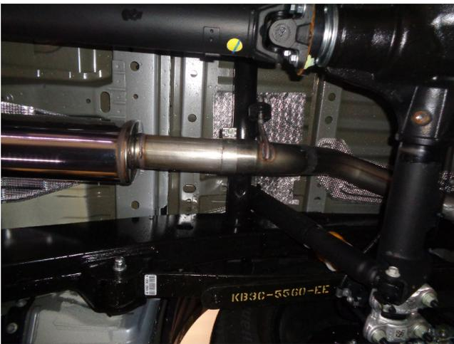
**Step 3.** Next loosely attach the Tailpipe Assembly to the Muffler Assembly using the supplied clamp. Engage the welded hanger to the rubber insulator.
