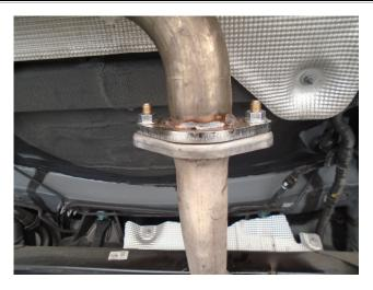
**Step 2:** Begin Installing the new MagnaFlow system by attaching the inlet pipe to the OE outlet using the supplied fasteners and gasket.
