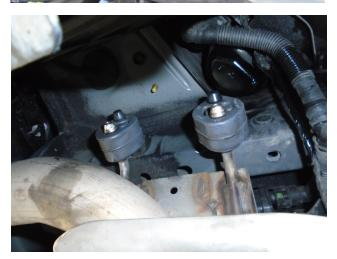
**Step 1:** To remove the OE muffler assembly unfasten the hardware at the flange. While supporting the muffler extract the hangers from the rubber insulators (retain rubber insulators as they will be reused).
