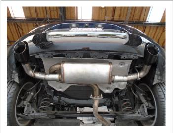
Once a final position has been chosen for the new exhaust system, evenly tighten all clamps from front to rear using the torque specifications on page one of the instructions. Inspect all fasteners after 25-50 miles of operation and re-tighten if necessary.
