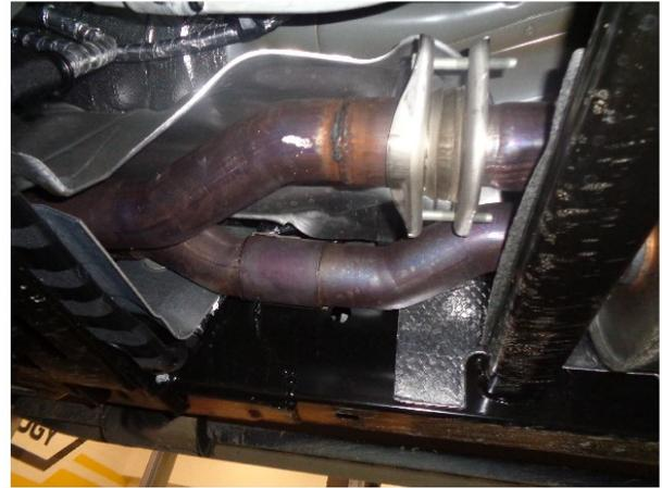
**Step 3.** Finally remove the OEM inlet muffler assembly by unbolting the inlet at the driver side flange junction and loosening the band clamp on the passenger side inlet pipe. Remove the inlet muffler assembly. You are now ready to install your new MAGNAFLOW exhaust system.
