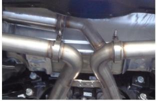
**Step 4.** Next install the passenger side Extension/Resonator Assembly followed by the driver side Extension pipe using supplied V-Clamps.
