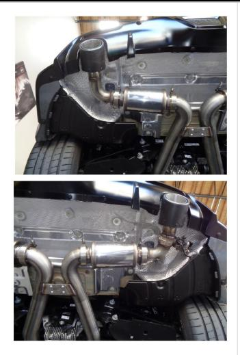
**Step 5.** Install the Muffler Assemblies (or Delete pipes) to the Extension Assemblies then attach the Tip Assemblies to the Mufflers using the supplied V-Clamps. Finish the installation by loosely attaching the MagnaFlow bracket between the Extension Pipes. Re-attach the valve wiring and OE cross brace.
