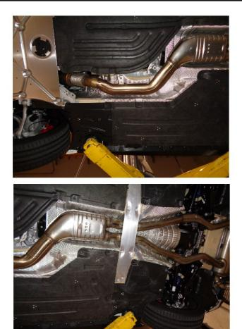
**Step 1.** To remove the OEM system first unplug the electrical connector at the exhaust valve located on the passenger side Tail Pipe. Begin by removing the cross brace then unbolt the mounting bracket and loosen the clamp at the exhaust inlet. Remove all welded hangers from the rubber insulators and remove the exhaust. Do not damage the fasteners or rubber insulators as they will be used to install the new MagnaFlow system.
