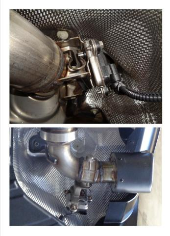
**Step 2.** Once the exhaust is off the vehicle remove the valve motor from the muffler assembly and transfer it over to the new exhaust valve assembly using the factory hardware.
