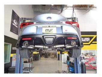
**Step 6.** Once a final position has been chosen for the new exhaust system, evenly tighten all clamps and fasteners, from front to rear, using the torque specifications on page one of the instructions. Inspect all fasteners after 25-50 miles of operation and re-tighten if necessary.
