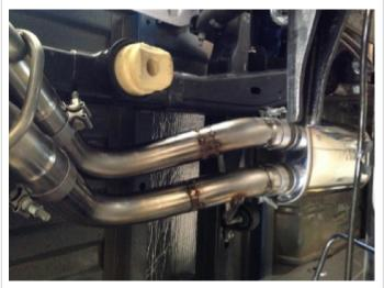
Step 4. . Install both the Over Axle Pipe Assembly and Tail Pipe Assembly using the supplied 2.50" clamps. Locate the welded hangers to the OEM rubber insulators.
