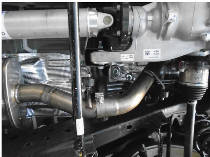
**Step 5.** Next loosely attach the Y-Pipe Assembly to the Muffler Assembly using the supplied clamp. Engage the welded hangers to the rubber insulators.
