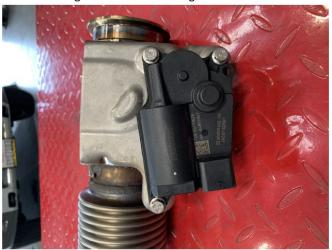
**Step 18.** Remove the three screws attaching the valve motor to the OEM valve. Remove the valve motor and heat shield.
