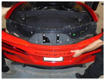
**Step 31.** All clamps and fasteners may now be tightened to the specs on the first page of this document. Reconnect the tail lights and reinstall the rear bumper, valance and wheel well covers in the reverse order of the removal process. Reinstall all underbody panels in reverse order of installation.
