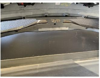
**Step 30.** Install the Rear Fascia Heat Shield by removing [4] bolts attaching the mesh. Locate the holes in the heat shield and secure using the OE screws.
