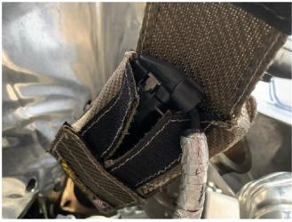
**Step 25.** Reconnect both electrical connectors to the valve motors. Close the Heat Blanket.
