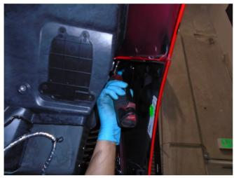
**Step 9.** Remove the 7mm hex bolts, two per side.
