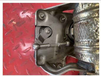
**Step 17.** Now that the OEM exhaust is removed from the vehicle the valve motor control arm will need to be removed. Uncouple the ball from the socket of the linkage arm. Next, remove the screw attaching the control arm using a T-25 Torx bit.
