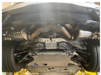
**Step 30.** Loosely install both Muffler/Tip asseblies to the X-Pipe Assembly. Loosely secure using the supplied clamps. Engage the welded hangers to the rubber insulators.
