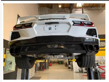
**Step 32.** The install process is now complete. After approximately 50 miles re-tighten all fasteners and clamps to the torque setting in the first page of this document.
