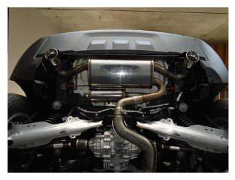
**Step 3** Next, attach the Muffler Assembly to the Inlet Pipe using the supplied 2.25" clamp. Engage the welded hangers to the rubber insulators. It may be necessary to loosen the pipe junction between the catalytic converter and the OE resonator to allow for proper tip alignment.
