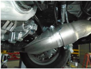
**Step 2**: Begin installing the new exhaust system by attaching the specific Inlet Pipe (2.0L or 1.5L engine) to the cut OE outlet using the supplied 2.18/2.36 clamp. Use the supplied hose clamp to re-attach the heatshield if necessary.
