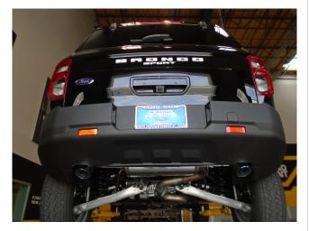
Once a final position has been chosen for the new exhaust system, evenly tighten all clamps from front to rear using the torque specifications on page one of these instructions. Inspect all fasteners after 25-50 miles for operation and re-tighten if necessary.
