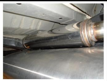
**Step 6:** When using the NDT chamber, mount it above the muffler as shown. Be sure to leave at least 1/2" of clearance between both components.
