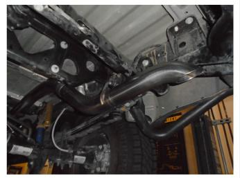
**Step 8:** Install the Tail Pipe to the Over Axle Pipe outlet using the supplied clamp. Engage the hanger to the OE rubber insulator.
