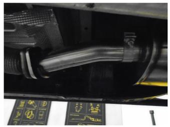
**Step 4:** Begin Installing the new system by attaching the inlet pipe to the Catalytic Converter outlet using the OE hardware. **NOTE: 15-17 vehicle will use the longer inlet and 18-21 will use the shorter inlet.**
