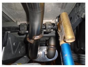
**Step 7:** Install the Over Axle Pipe to the Muffler outlet using the supplied clamp. Engage both hangers to the OE rubber insulators.
