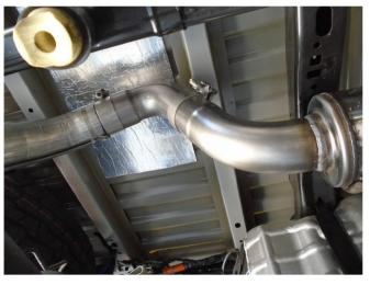
**Step 7:** For 2021 models slip the Muffler Assembly outlet to the supplied Outlet Pipe with the 3" clamp. Then attach the cut tail pipe using the 3.18" clamp. Loosely secure both clamps.
