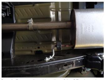
**Step 3:** Remove the mid section of the OE exhaust by loosening the clamp forward of the muffler shown. Then disengage the hangers from the rubber insulators. Be sure to not damage the rubber insulators as these will be used for the new MAGNAFLOW Muffler.
