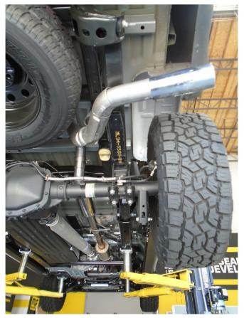
**Step 8:** Once a final position has been chosen for the new exhaust system, evenly tighten all clamps. Inspect after 25-50 miles for operation and re-tighten if necessary.
