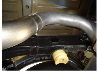
**Step 6:** For '15-'20 models slip the Muffler Assembly outlet to the cut OE muffler pipe. Loosely secure with the supplied clamp.
