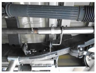
**Step 4:** Install Inlet Pipe for your application. The smaller inlet diameter is for 2015 - 2020, the larger is for 2021. Loosely attach the inlet of the Inlet Pipe fo the vehicles inlet pipe outlet using the OE clamp.
