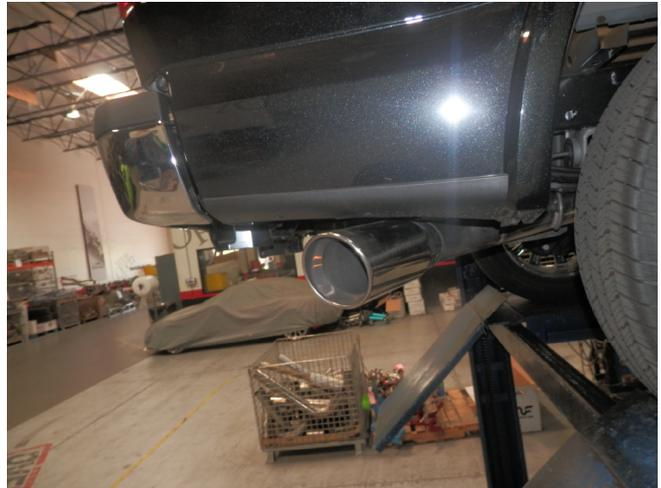
**Step 8.** Once a final position have been choden for the new exhaust system, evenly tighten all clamps from front to rear using the torque specifications on page one of these instructions. Inspect all fasteners after 25-50 miles of operation and re-tighten if necessary.
