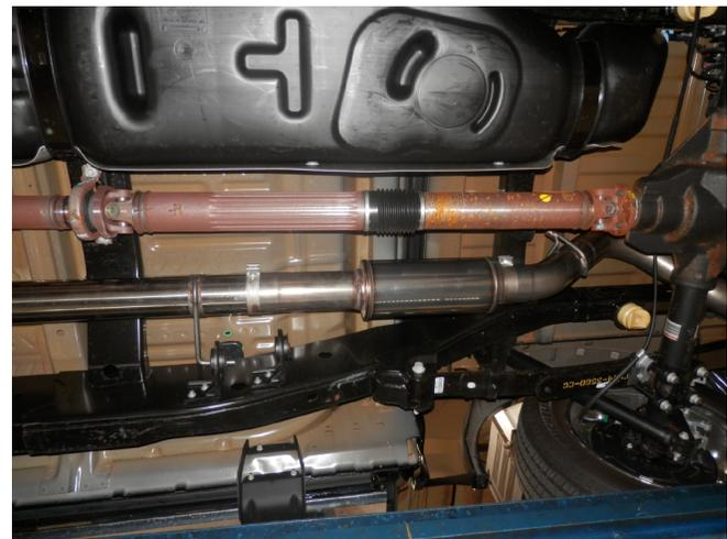
**Step 5.** Next loosely install the Muffler Assembly to the Inlet Pipe Assembly or Extension Pipe using the supplied clamp. Engage the welded hanger to the rubber insulator.
