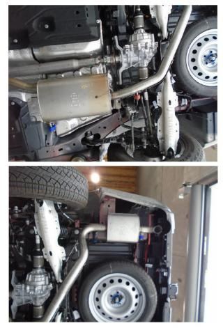
**Step 2:** With the system supported, working front to rear disengage the hangers from rubber insulators and remove the OE system. Do not discard or damage the rubber insulators as they will be used to install the new system.
