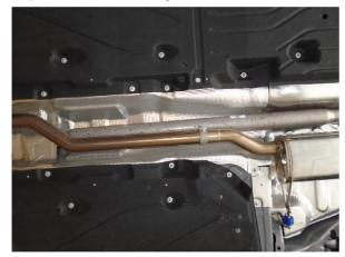
**Step 4:** Attach the Muffler Assembly to the Inlet Pipe
