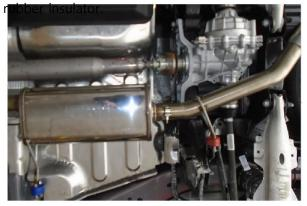
**Step 5:** Attach the Muffler and Mid-Pipe Assemblie using the provided 2.50" Clamps. Fit hangers into rubber insulators.
