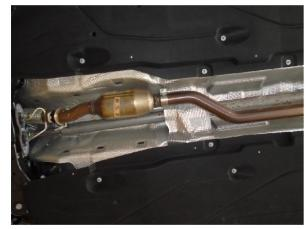
**Step 3:** Begin installation of your new MAGNAFLOW system by attaching the Inlet Pipe to the cut outlet of the converter using the supplied 2.36" clamp. Keep all clamps loose until final adjustment.
