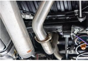
**Step 3:** Install new MagnaFlow Muffler by first sliding the outlet onto the OE System and then bolting the MagnaFlow flange to the OE flange using the OE fasteners.
