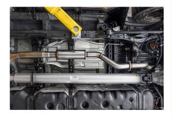
Finish by inserting the hangers into the rubber insulators and securing the supplied 3.00" clamps. Once a final position has been chosen for the new exhaust system, evenly tighten all clamps and bolts from front to rear. Inspect all fasteners after 25-50 miles for operation and re-tighten if necessary.
