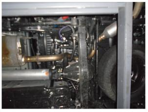
Remove the OE Muffler by loosening and removing the bolts at the outlet flange. Then disengage the hangers from the rubber insulators. Do not damage the rubber insulators or discard the fasteners as these will be used for the new MagnaFlow Muffler.
