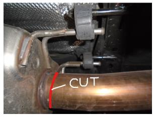
Begin removal of the OE muffler by marking cut point a 1/2" to the rear of OE Muffler as shown in photo below. Then cut the OE Exhaust at that cut point.
