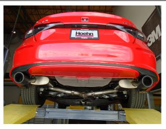
**Step 6:** Once a final position has been chosen for the new exhaust system, evenly tighten all clamps from front to rear using the torque specifications on page one of these instructions. Inspect all fasteners after 25-50 miles for operation and re-tighten if necessary.
