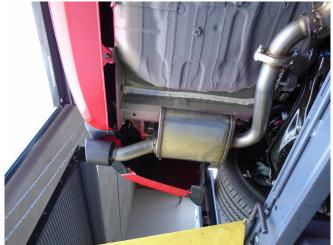
**Step 5**: Loosely attach both driver and passenger side Muffler Assembly flanges to the Y-Pipe Assembly. Secure with the supplied gaskets and hardware. Engage welded hangers to rubber isolators.
