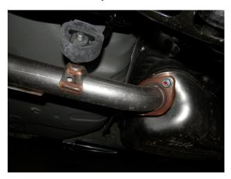
**Step 2.** Unbolt the drivers side OEM muffler assembly at the flange junction. Disengage all welded hangers from the rubber isolators. The OEM exhaust system may now be removed.
