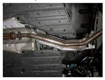
**Step 4.** Next attach the Y-Pipe Assembly to the Inlet Resonator Assembly by fastening the flanges using the supplied gasket and hardware.
