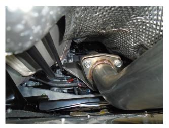
**Step 3.** Begin installation of your new MAGNAFLOW system by attaching the Inlet flange of the Inlet Resonator Assembly to the catalytic converter outlet using the OEM fasteners. Engage the welded hanger to the rubber isolator. Keep all fasteners and clamps loose until final adjustment.
