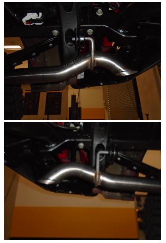
**Step 5.** Complete the installation by attaching both Tailpipe Assemblies to the Y-Pipe Assembly using the Supplied 2.50" clamps and fitting the hangers into the rubber insulators.
