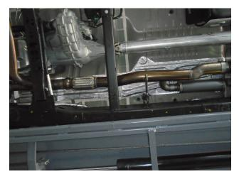
**Step 3.** Only the Crew Cab Long Bed configuration will require the supplied 12.5 Extension Pipe, Install this to Inlet Pipe Assembly if required using the supplied 3.50" clamp then attach the Muffler Assembly to the Extension Pipe. If the 12.5" Extension Pipe isn't used attach the Muffler Assembly directly to the Inlet Assembly with a supplied 3.50" clamp.
