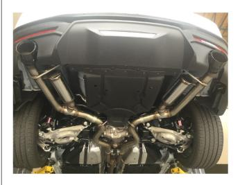
**Step 4.** Finish the initial installation by fitting the Muffler Assemblies onto the Mid pipe Assemblies using the supplied 3.00" clamps and inserting the hangers into the rubber insulators.
