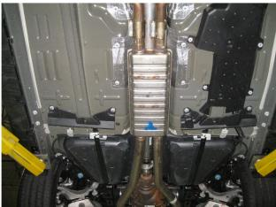
**Step 1.** Start removing the OEM exhaust system by loosening the clamps located in front of the resonator. Next working front to rear extract the hangers from the rubber insulators and remove the OEM system. Retain insulators and clamps as they will be used to install the new system.
