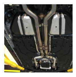
**Step 3:** Begin installation of the new system by loosely attaching the H-Pipe Assembly to the outlets using the OEM clamps. Leave all clamps loose until final adjustment.
