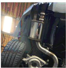
**Step 5:** Finish the initial installation by fitting the Muffler Assemblies onto the Mid pipe Assemblies using the supplied 3.00" clamps and inserting the hangers into the rubber insulators.
