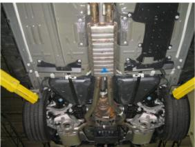
**Step 2:** Begin removing the OEM exhaust system by loosening the clamps located in front of the resonator. Next working front to rear extract the hangers from the rubber insulators and remove the OEM system. Retain insulators and clamps as they will be used to install the new system. Remove actuators from OEM exhaust and install on new rear muffler assemblies. Reuse OEM fasteners, heat shield and spring.
