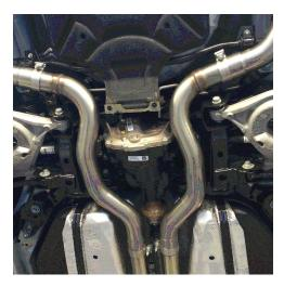
**Step 4:** Next attach the Mid Pipe Assemblies to the H-Pipe using the supplied 3.00" clamps and fitting the hangers into the rubber insulators.
