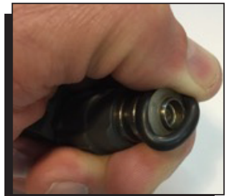
Figure 2 - Installation of MSD O-Ring
