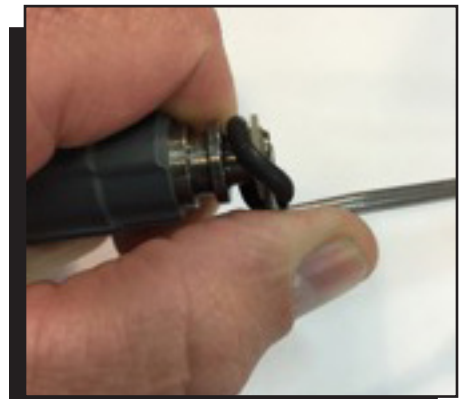
Figure 1 - Removal of original O-Ring
