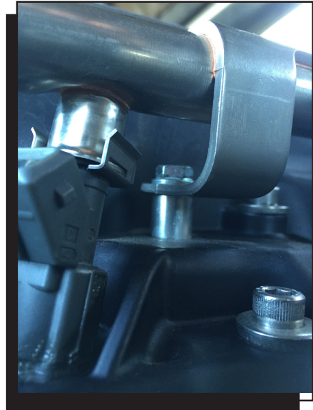
Figure 3 - Fuel Rail Spacer and Flange Head Bolt
