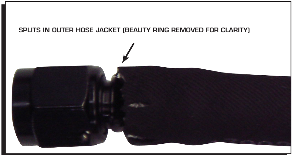
Figure 8 Improperly Installed Push-Lock Fitting
