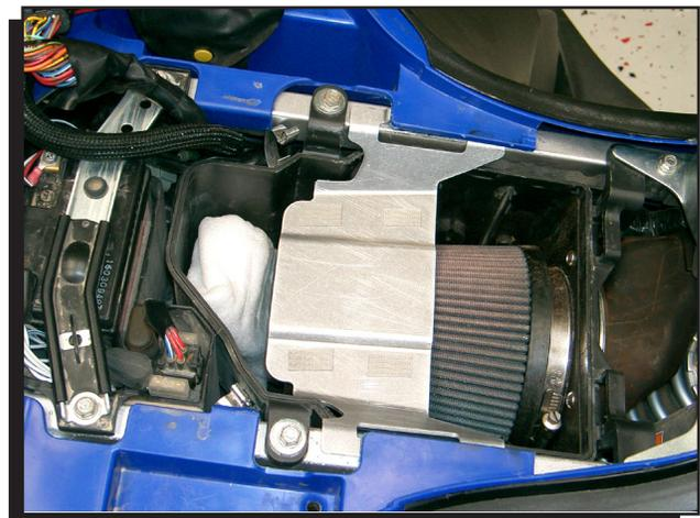
Figure 2 Hook Bracket and Velcro Install.
