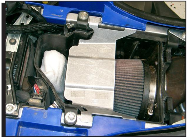
Figure 1 Bracket Install.
