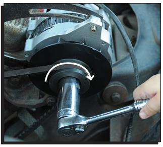
Figure 3 Checking Belt Tension.
