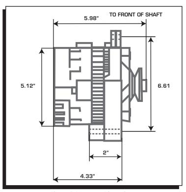
Figure 2 Alternator Dimensions.
