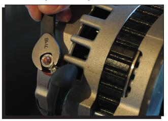
Figure 4 Installing the Charge Wire.
