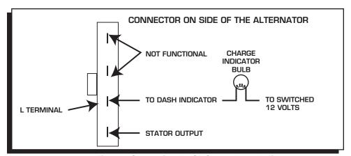
Figure 5 Connecting the OE Charge Lamp Indicator.
