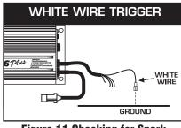
Figure 11 Checking for Spark with the White Wire.
