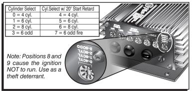
Figure 2 Programming the Number of Cylinders.
