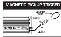
Figure 12 Checking for Spark with the Mag Pickup.
