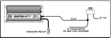
Figure 5 Wiring the 2-Step Rev Limit.
