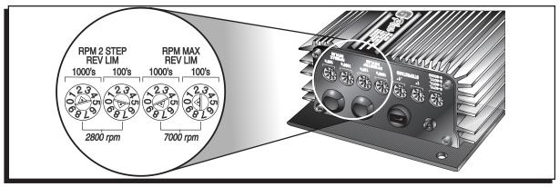
Figure 4 Adjusting the Rev Limits.
