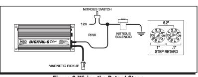
Figure 6 Wiring the Retard Stage.
