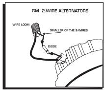
Figure 10 Installing the Diode to a 1973-1983 GM Vehicle.
