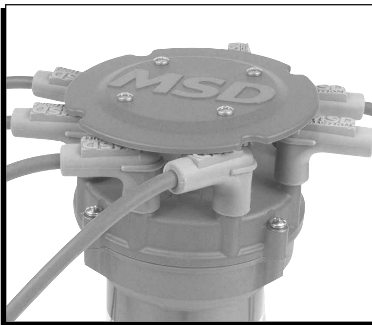
Figure 7 Installing the Wire Retainer.
