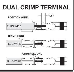
Figure 2 Crimping a Dual Crimp Terminal.
