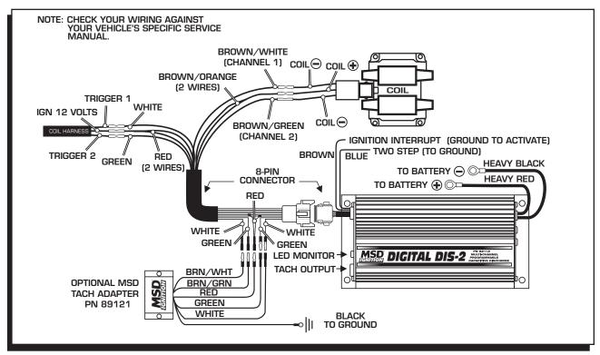
Figure 2 Typical Installation with an MSD DIS-2 Ignition.
