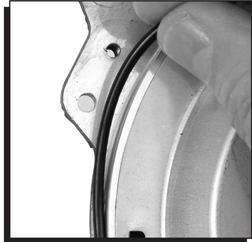
Figure 2 Installing the Distributor-to-Isolator Seal.
