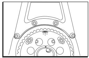
Figure 1 Installing the Distributor Bracket.
