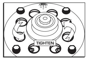
Figure 2 Installing the Timing Belt Pulley.
