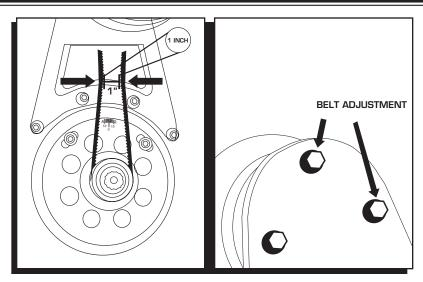
Figure 3 Adjusting the Belt Tension.
