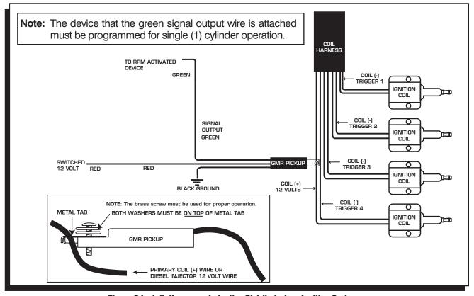
Figure 2 Installation on an Inductive Distributorless Ignition System.
