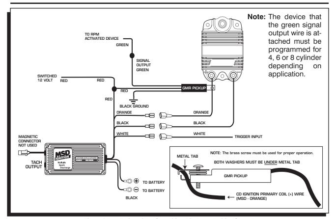
Figure 1 Installation with a Capacitive Discharge Ignition Control.
