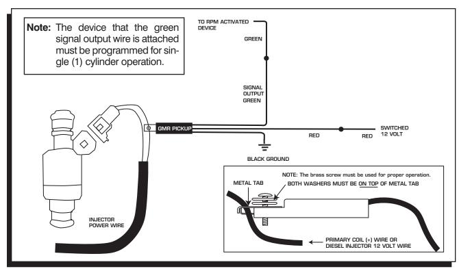
Figure 4 Installation to a Diesel Injector.
