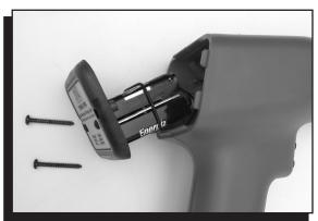
Figure 1 Replacing the Six AAA Batteries.
