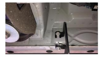
**Step 6:** Next, tighten all hardware beginning with the lower mounts first then the upper mounting locations. **Step7:** Tighten (x3) brackets at the main tube.
