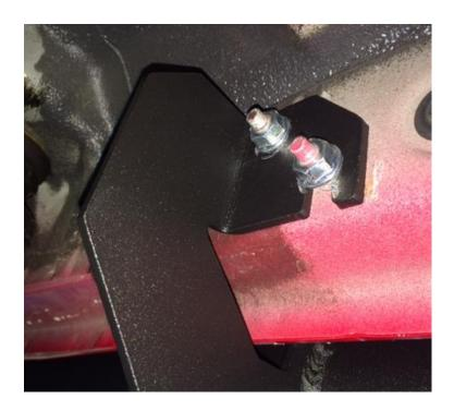
**Step3:** After final alignment torque all hardware to 15-20 ft/lbs.
