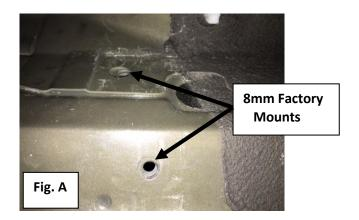
**<u>Step 2</u>**: Starting with the driver's side, lift step up into position aligning the step bracket with the 8mm OE mounts. **(Fig. B)**
