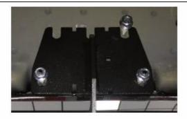
**Step 5:** After finial adjustment, tighten (x3) bracket to (20 ft./lbs of torque.)
