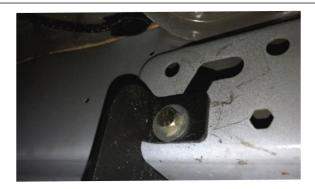
**Step 8:** Insert the black zinc M8 flanged bolts and flanged nuts in the pinch weld holes and leave loose for now.
