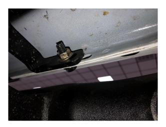
**Step 9:** Begin tightening the lower attachment points starting with the rear bracket working your way up to the front bracket. **( 20ft/lbs )**
