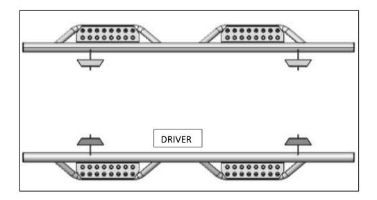
**Step 1:** Starting with the Driver Side. Remove all 8mm flange nuts from the 8mm factory threaded studs to remove the OE running boards.
