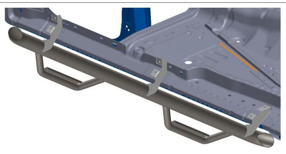
**Step 6.** Tighten the three lower bolts first following with the three upper bolts. **Step 7.** Next, tighten brackets (x3) at the main tube.
