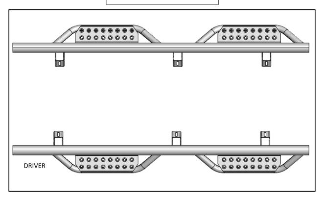
**Step 2.** Install the (x6) mounting brackets to each attachment point on the main tube using the supplied M10x25 carriage bolts, M10 hex nuts and leave loose for now.
