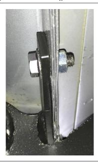
**Step. 7:** After finial positioning, completely tighten all (x6)  $\frac{1}{2}$ " -20 x  $\frac{3}{4}$ " in the pinch weld attachment.
