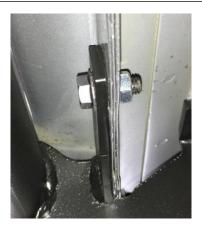
**Step 10.** Next, tighten the remaining hardware that attaches the bracket to the upper body mount.
