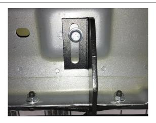
**Step 11:** After finial adjustment, tighten all three brackets at the main
