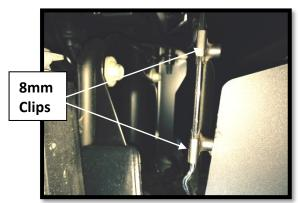
**Step 2:** Align the two Base brackets to the 8mm clip mounts and fasten using the supplied 8X 20mm hex head bolts and washers. Loosely tighten at this time.
