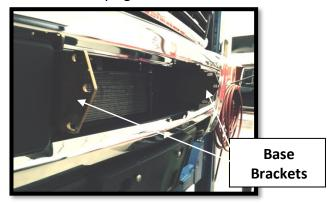
**Step 3:** Align the Light bar brackets with the Base brackets and fasten with the supplied 8 X 20mm button head bolts, nuts, and washer and loosely tighten.
