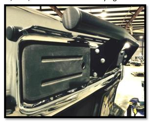
**Step 4:** Once the light bar is aligned to desired position, tighten all hardware. Your install is now complete.
