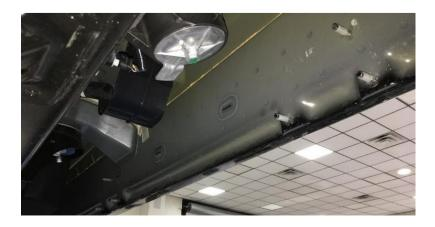
**Step 3:** On the inside rocker panel there will be three-attachment point consisting of three 8mm studs coming out from the panel. These studs may be covered in paint and will need to be cleaned before the installation.
