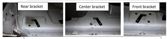
U-clip positioning. NOTE: Clips will also face forward for passenger side.
