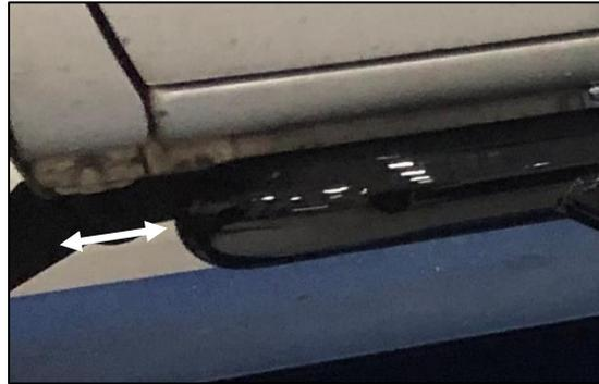
**Step 4:** Next, make a mark through each bracket mounting location onto the center of the pinch weld. Transfer your marks to the out-side of the pinch weld to center your holes that will be drilled.
