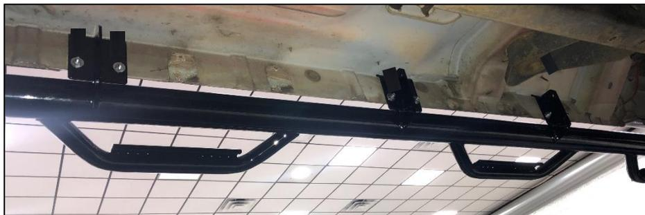
**Step 3:** The front tip of the tube will go approximately **2 ½"** behind the fender well opening.
