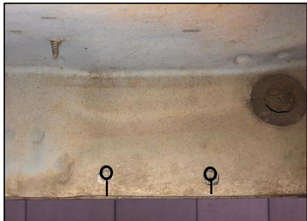
**Step 5:** After you have your holes marks transferred to the pinch weld on the out- side of the vehicle, take a center punch to mark the centers for drilling. Drill each hole using a 3/8" drill bit. **NOTE:** A 3/16" pilot hole is recommended.
