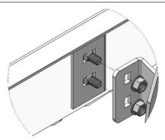
**Step 3**: Look on the underside of the body and locate the factory supplied mounting positions. **NOTE:** Some vehicles require the use of speed clips and nuts, which are supplied with the hardware kit.
