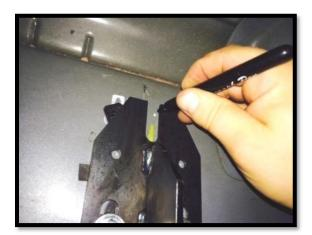
**<u>Step 7:</u>** Remove Nerf Step and set aside. Next, slide the additional 3/8 threaded clip from the upper rectangle hole and align with the "U" shaped mark. Make a mark through the threaded part of the clip.
