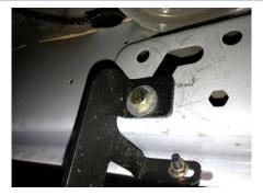
**Step 10:** Next, adjust the step assembly up/down and front/back to level out the step rail with body panel and then tighten step to brackets at 20 ft. /lbs.
