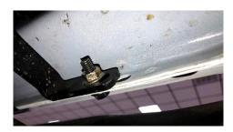
Step 8: Begin tightening the lower attachment points starting with the rear bracket working your way up to the front bracket. (20ft/lbs)
