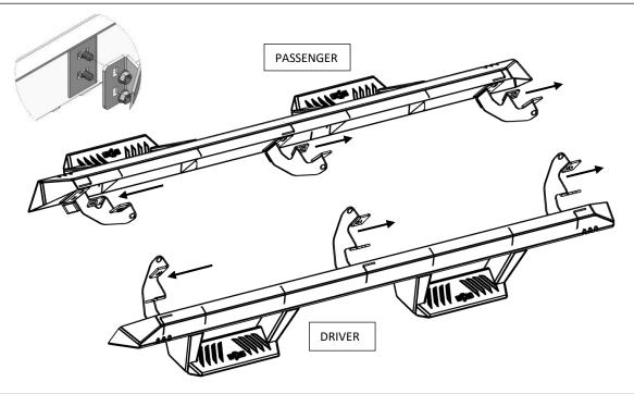
**Step 3:** Remove any factory running boards or steps and discard. **Step 4:** Next, locate the mounting holes underneath the body and remove the factory tape from the three locations.
