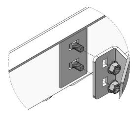
NOTE: Larger bracket will attach towards the front of step rail in the first position.
