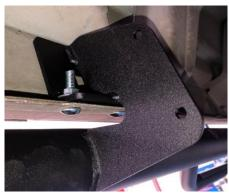
**Step 4:** After finial adjustment, tighten all hardware to 17-20 ft./lbs. of torque. Step 5: Repeat with passenger side.
